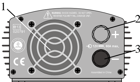
Figure 5 DC Panel on the XPower 500
