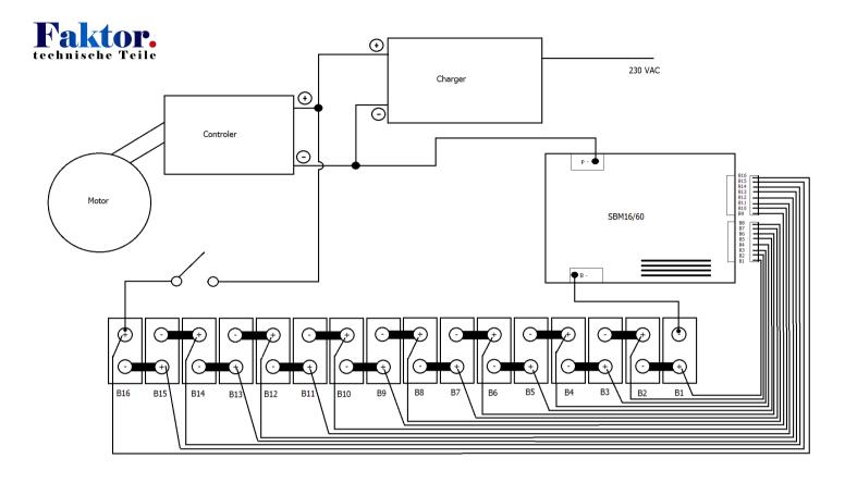
This schema is applicable to every SBM modules with difference in number of monitored cells.
