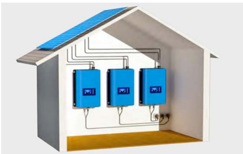
Fig 2. Multiple inverters can be connected in parallel to create a bigger system. Plug and play installation
