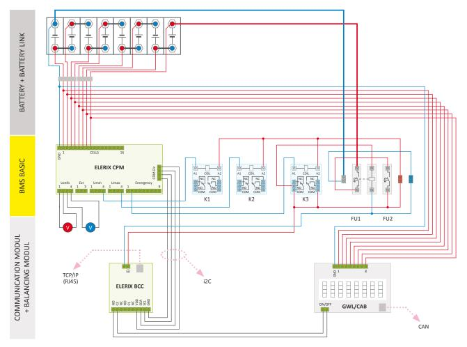
High-impedance voltmeters can be connected to the "green" outputs on the CPM to get basic information on the battery status. They transmit the value of the cell with the lowest (Umin - red) and the highest (U max - blue) voltage from the entire module. "Green" IQ BUS outputs provide information on voltage in the i2c protocol, which can be used for the connected customer device (open source).
