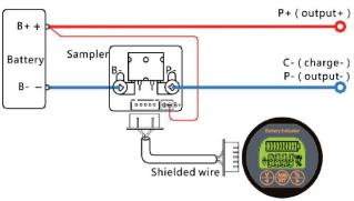
★ Connection diagram of 100A/350A sampler :
