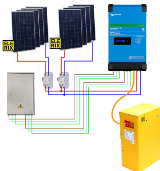
Single-phase hybrid PV plant
