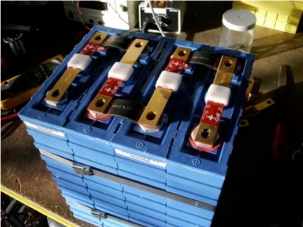
Lay out and bolt down all the cell modules and interconnectors.
