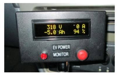
The BCU has two display modes, just press and hold the monitor button to toggle between them. This button may also be pressed to reset any error conditions.
