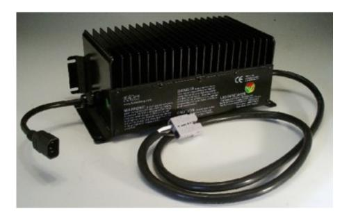
EV Power supplies a range of PFC chargers to suit LFP batteries. This type of charger can be permanently connected directly to to battery. It has a charge control cable that connects to the BCU charge control circuit. In this way the BCU can control charging directly and automatically without user intervention.
