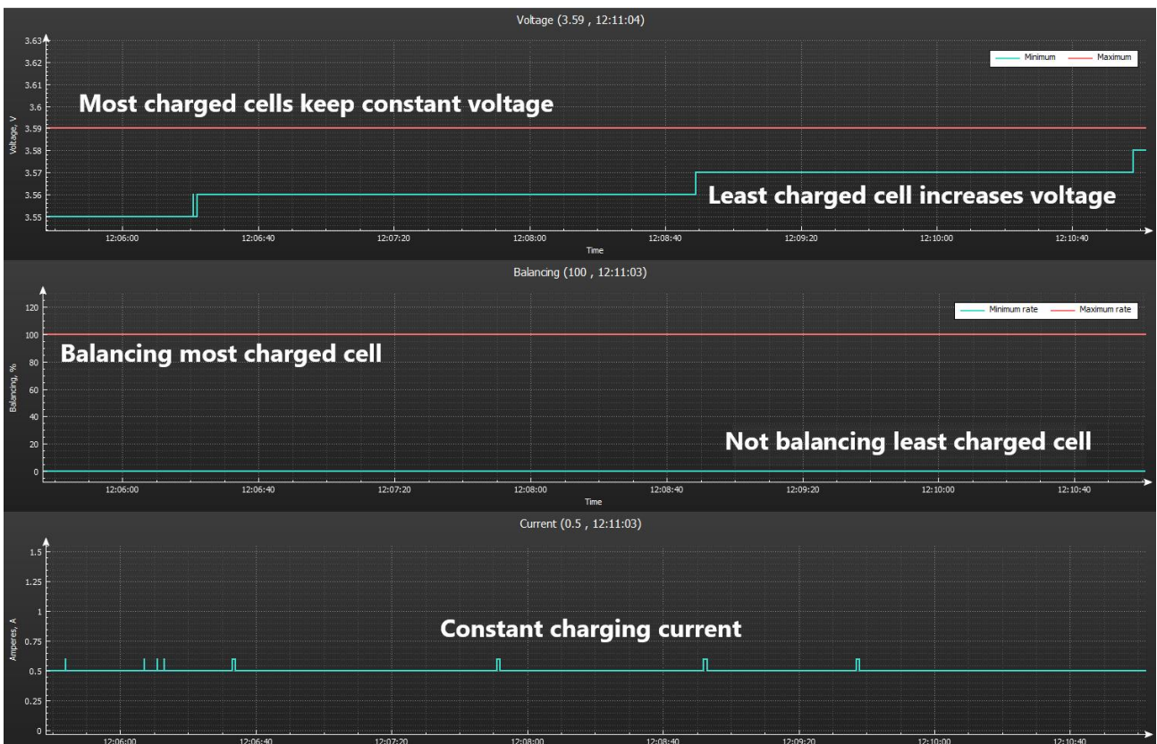
Figure 2.8 Charging algorithm end of charge logic
