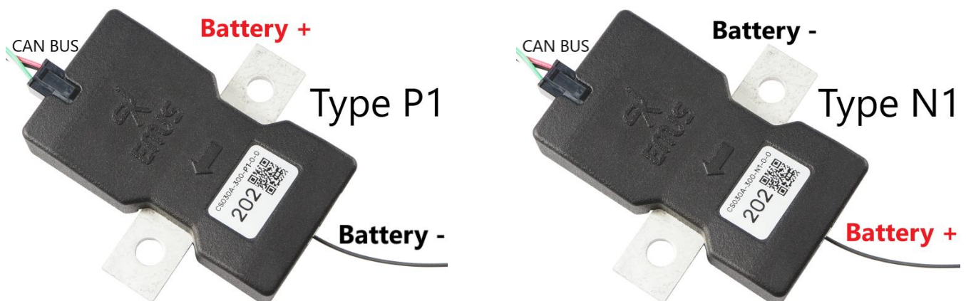
Figure 1.13 EMUS CAN current sensor installation types N1 and P1 respectively
