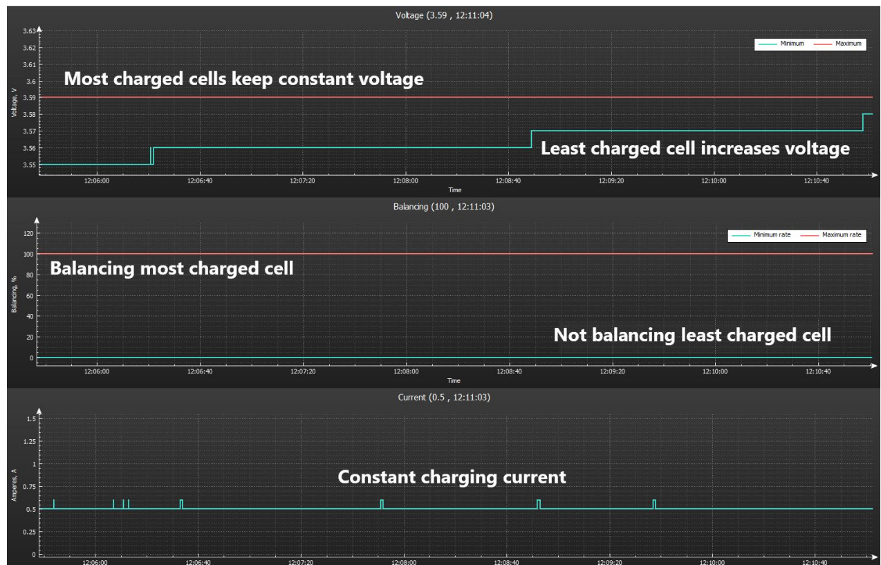
Figure 2.8 Charging algorithm end of charge logic
