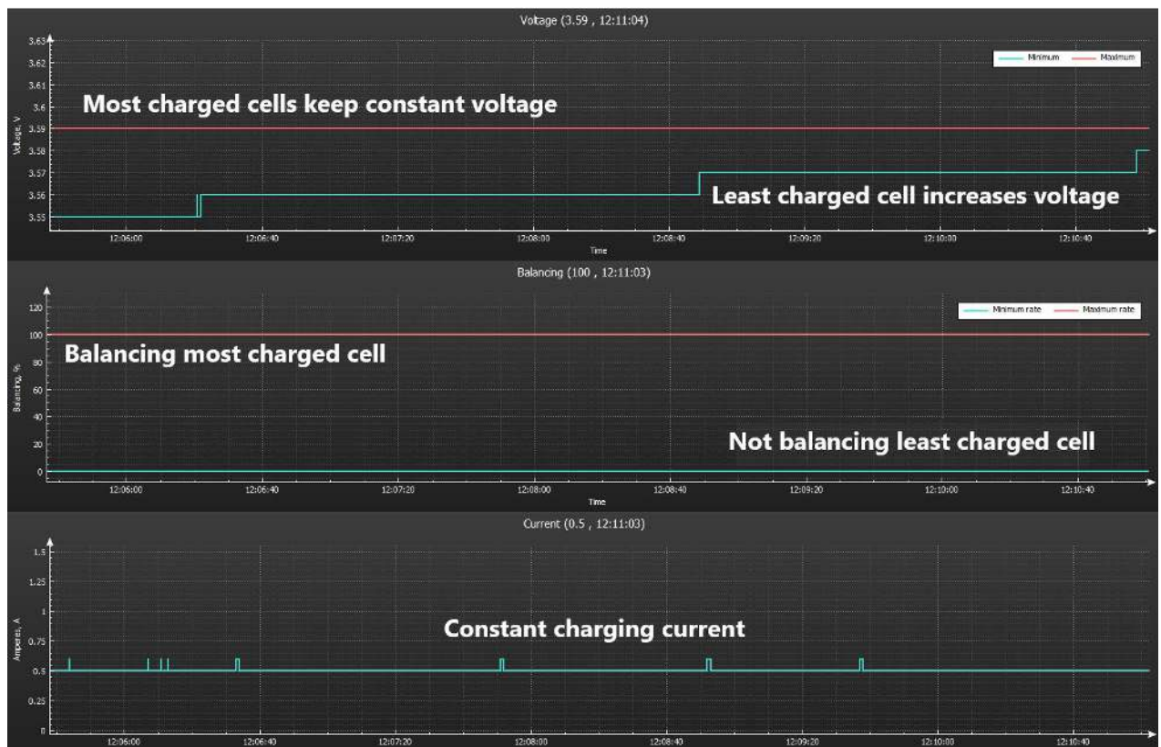
Figure 2.8 Charging algorithm end of charge logic
