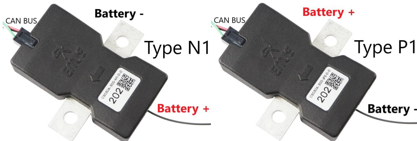
Figure 2. CS030A type N1 and P1 installation respectively
