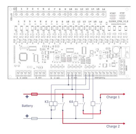
Connect the high charge current via a standard single-coil relay, low charge current via a two-coil bi-stable relay. The 'Charge 1' high charge power will be disconnected 15 seconds after reaching Umax, and the 'Charge 2' low charge current will no longer be disconnected if the cell voltage drops below Umax again within 20 seconds.
