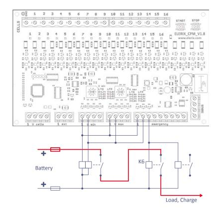
For each protection (Umin Umax Uemergency), it is advisable to use a separate relay for maximum battery protection. The combination of two or three pulse outputs per bi-stable relay reduces the quality of protection (possibility of contact bonding, coil or output failure, etc.). The combination of pulses can be used in justified cases; the electrical module structure makes it possible.
