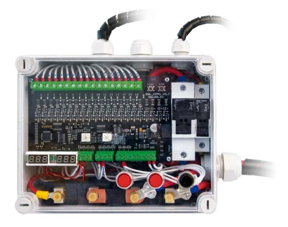
CELL PERFORMANCE MONITOR 4-16 cells LiFePO<sub>4</sub>/LTO
