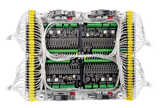
CELL PERFORMANCE MONITOR 4-16 cells LiFePO<sub>4</sub>/LTO
