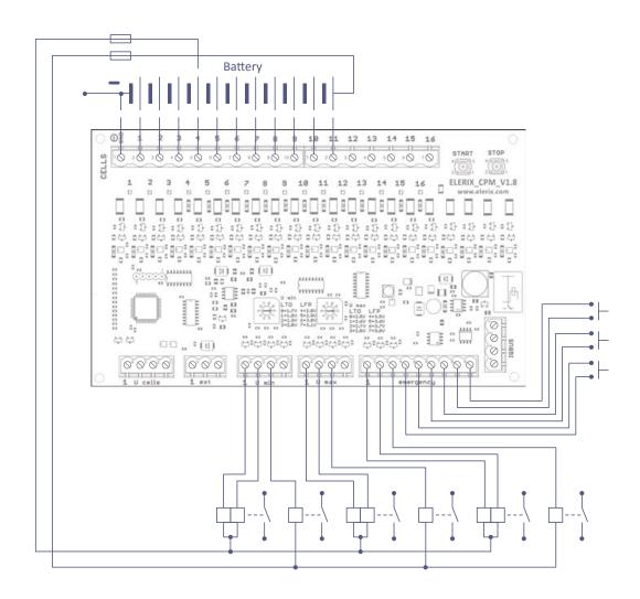
Any number of cells in the range of 4–16 can be connected; always from terminal 1 in the electrical sequence of the serial connection to the battery. A parallel battery cell connection is considered to be one cell.
