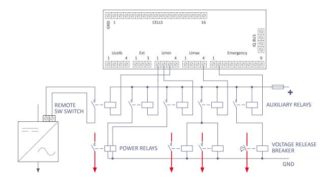
Switching power of relays coils and contactors may not exceed the switching range of CPM outputs defined in the product datasheet. For higher switching power use auxiliary relays.
