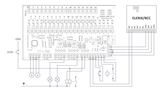
Control inputs of the standard relays (Umin 3 and 4, Umax 3 and 4, Uemerg 3) can be also used for signalization of the limit state. The bistable relays can be additionally controlled by GND impulse using the auxiliary button.
