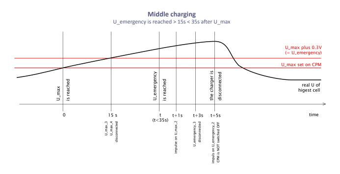
CELL PERFORMANCE MONITOR 4-16 cells LiFePO<sub>4</sub>/LTO
