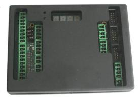
\*) **Note 1:** Output indication signals (connector A, pins 6 ÷ 9) are in the default version analog (connection of analog displays). For outputs AD2, 3 and 4 it is possible to set by jumpers U3 the output voltage (either 0 up to 3.3V or 0 up to 10V) by jumper between connectors "A" and "C".
