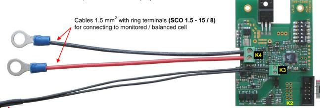
Module with conductors and ring terminals (SCO 1.5 -15/8) for connection to the monitored cell and temperature sensor (TEMP-SW 20) to measuring the temperature of that cell.
