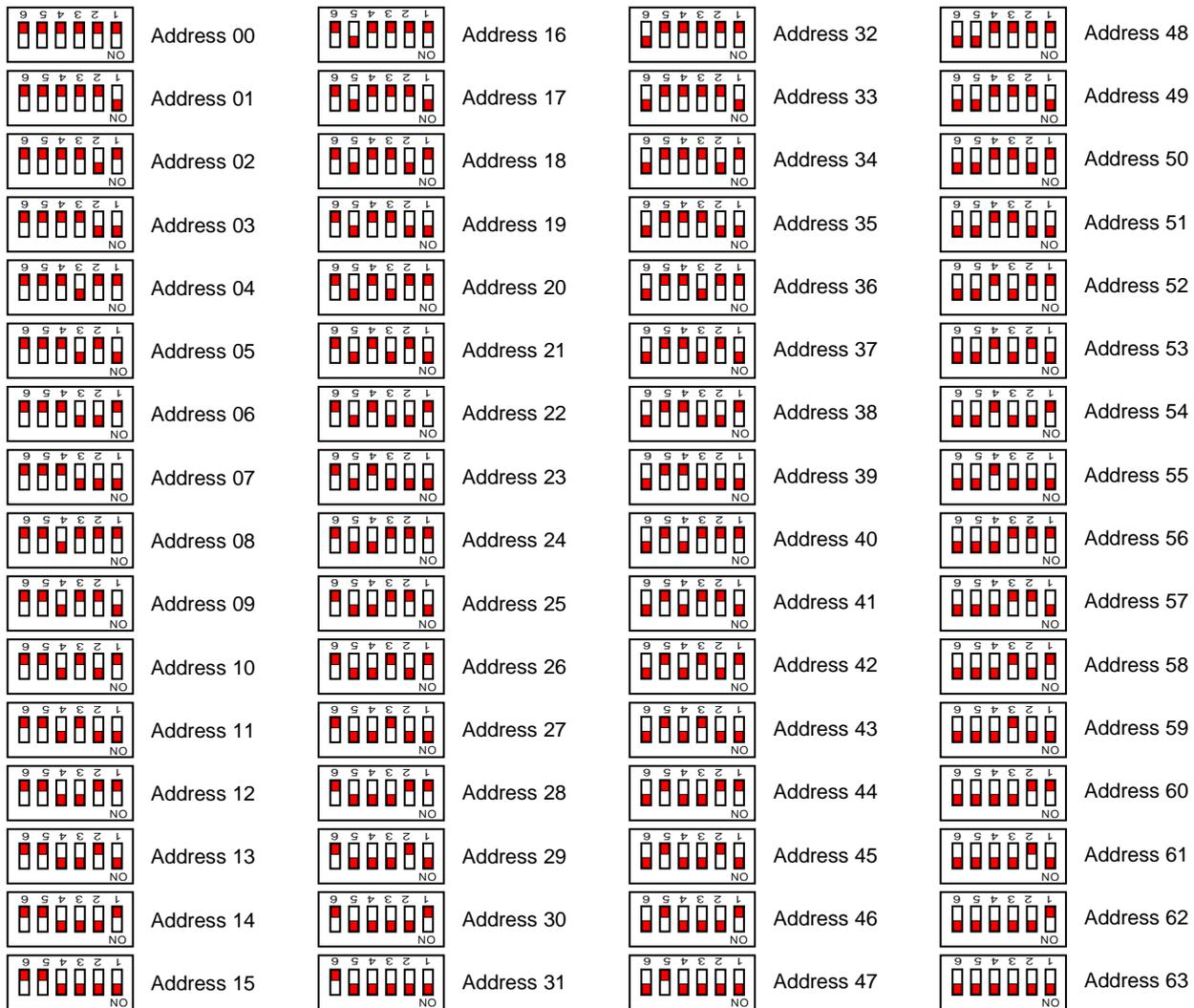
Essentially it does not matter which module, i.e. having which specific address, each cell has assigned to it. The easiest arrangement when, for example, identifying a faulty cell or a cell in poor condition, it is best to assign the lowest cell number **1** (the closest to the battery pole) the address "00" and assign the rest of the cells in order from there, i.e. "01", "02", and so on.
