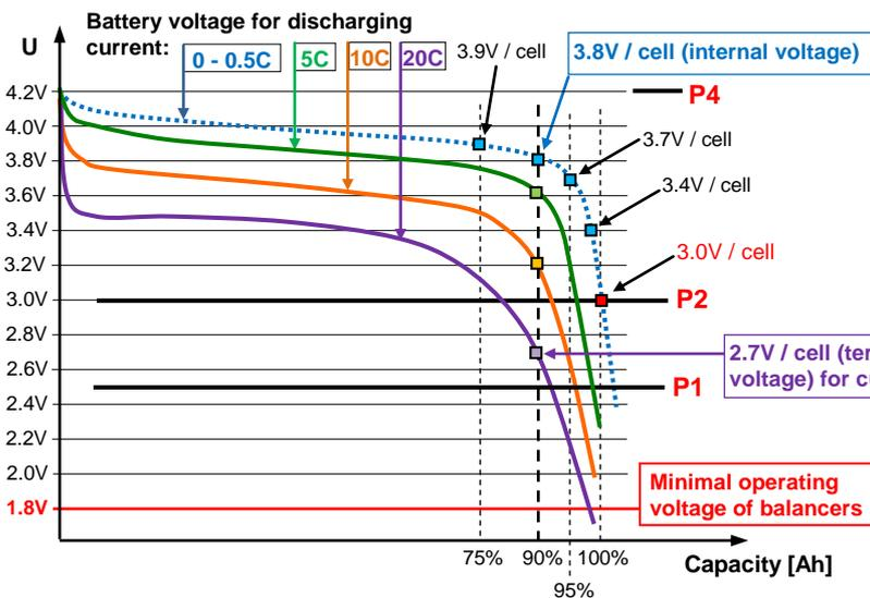
Because terminal voltage of the cell is **strongly depend on the current and internal cell resistance** (see picture on the left side), for evaluating the state of cells is used internal cell voltage, which are independent of the above variables and so eliminate their negative influence.
