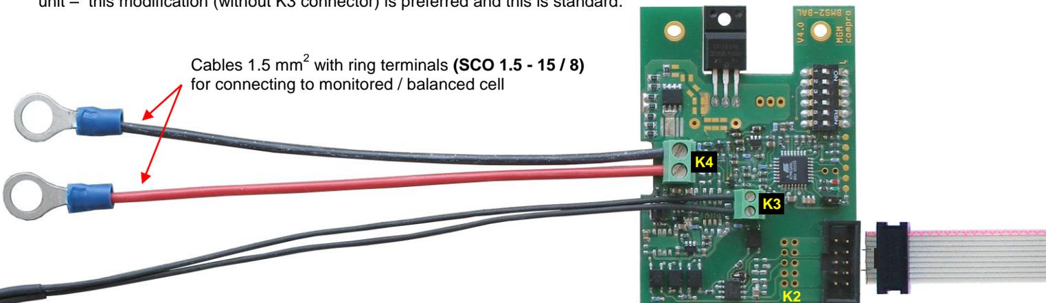
Module with conductors and ring terminals (**SCO 1.5 -15/8**) for connection to the monitored cell and temperature sensor (**TEMP-SW 20**) to measuring the temperature of that cell.
