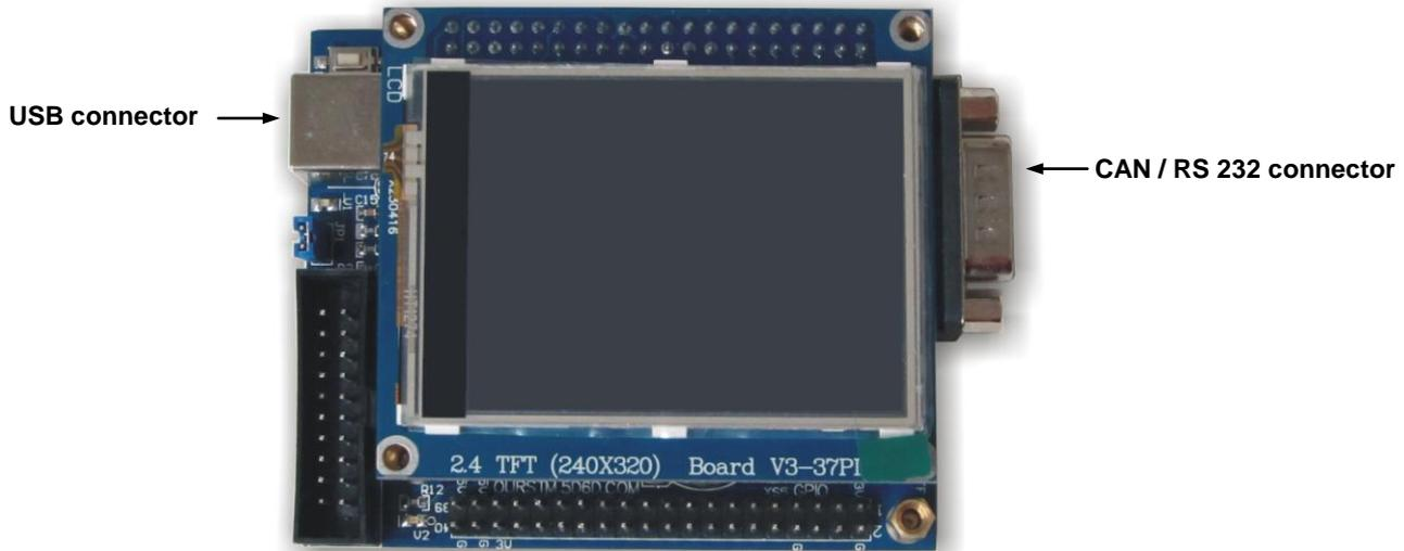
Display GWL 320 x 240 need external feeding 5V / 250mA. This is possible connect to "USB" connector or via communication connector. Using this connector and PC is possible change some display characteristics.
