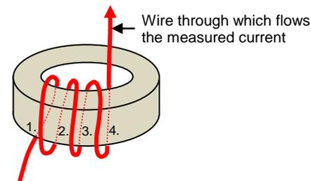
**Attention !** In some applications, can be problem the increased inductance by this method (winding it around turns around the coil you create higher inductance of this wire).
