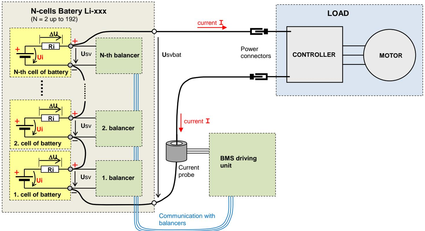
The minimum operating voltage of the balancing / measuring units (abbreviated balancers) is 1.8 V / cell. In this case, the terminal voltage of the cells it means, not the internal voltage. If the terminal voltage of cells drops for any reason under this limit, the corresponding balancer stops to measure and communicate with driving unit until the terminal voltage of the cell increases above 1.8 V.
