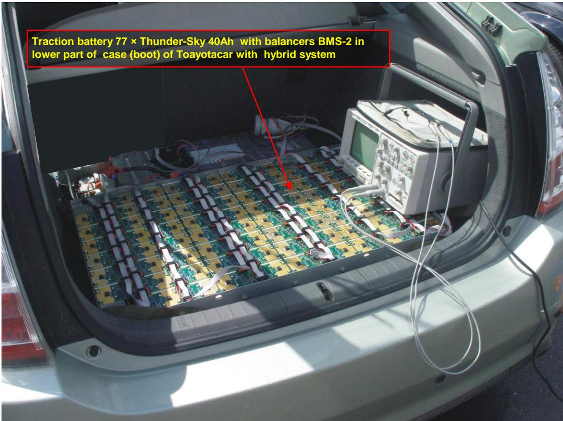
Traction battery 77 × Thunder-Sky 40Ah with balancers BMS-2 in lower part of case (boot) of Toyota car with hybrid system
