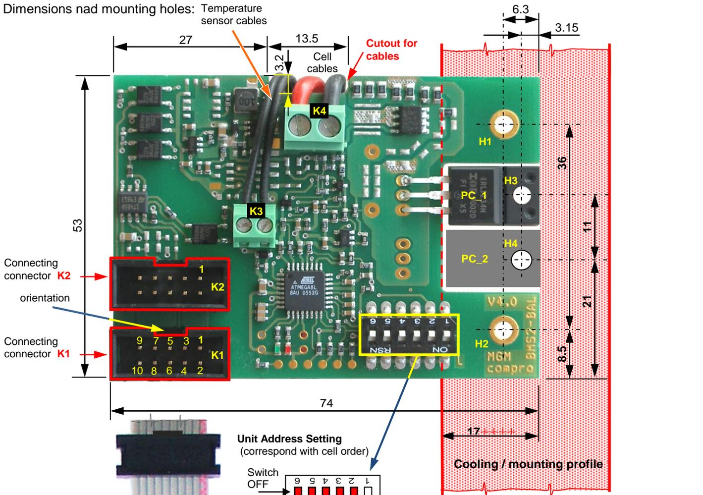
Power component PC\_x is mounted on to the cooler through silicone heat sink compound SP-100, DC 340, etc., screw M3x6 (M3x8) and spacer under screw.
