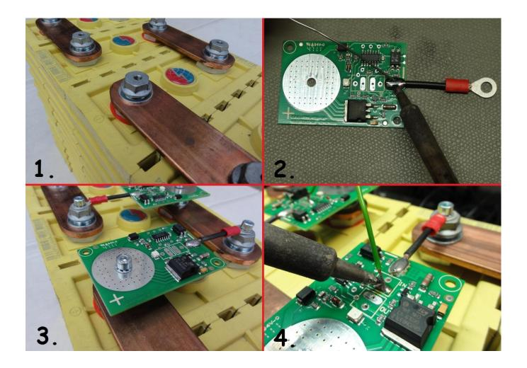
**WARNING :** be aware that your battery-pack contains a large amount of energy, which can be **potentially lethal**. Use isolated spanners, to prevent any short circuits. High inrush currents (causing sparks and ultra-high electro magnetic levels) can easily damage the electronic circuits.
