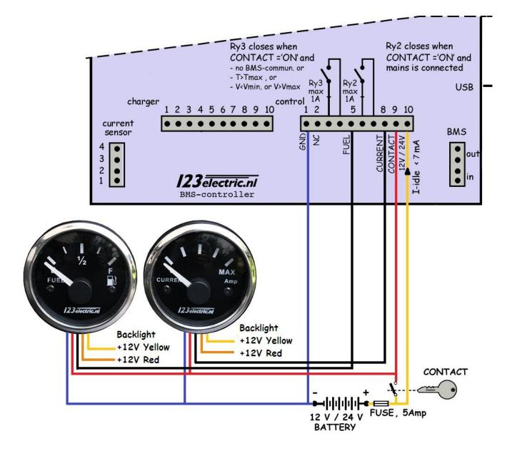
In the above schematic the "123electric" current- and fuel- gauges are drawn. Might you want to use your existing fuel gauges instead, you are free to do so. The BMS controller mimics a variable resistor between 0 and 240 Ohms and therefore practically any fuel gauge can be used. With the help of "analog gauge calibration" in the dashboard-software you should be able to linearize the reading of your gauge.
