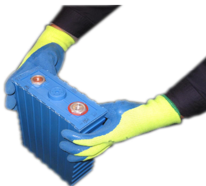
Picture 3.2.1.1: must put on insulating gloves
